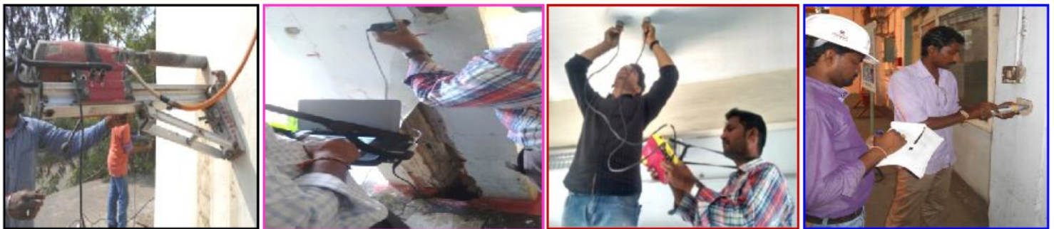
Our men at work! Performing Core test, Half Cell Potential test, Ultrasonic Pulse Velocity Test, and Rebound Hammer Test at NAVAL DOCKYARD
